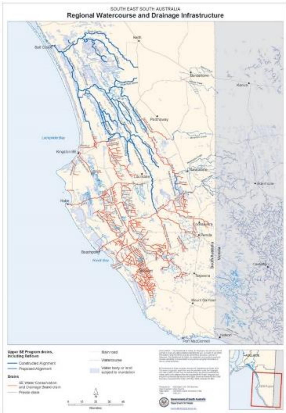
Figure 10: South East Drainage System Map
